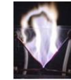
Gliding Arc setup designed for low temperature (45-65 °C) sterilization of metal coupons.
